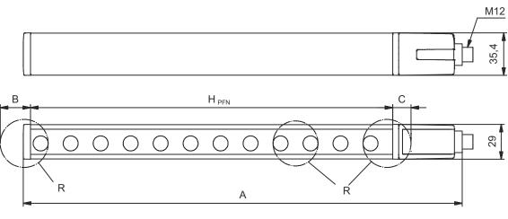
$H_{\rm PFE}$  Effective protective field height = 2490 mm  $H_{\rm PFN}$  Nominal protective field height = 2400 mm
