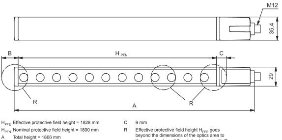
А В 19 mm Effective protective field height H<sub>PFE</sub> goes beyond the dimensions of the optics area to the outer borders of the circles labeled with R.
