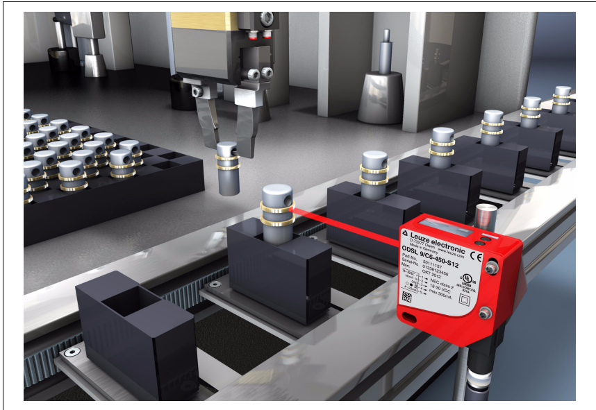
Bild 4.3: Application example: installation check with the ODSL 9
