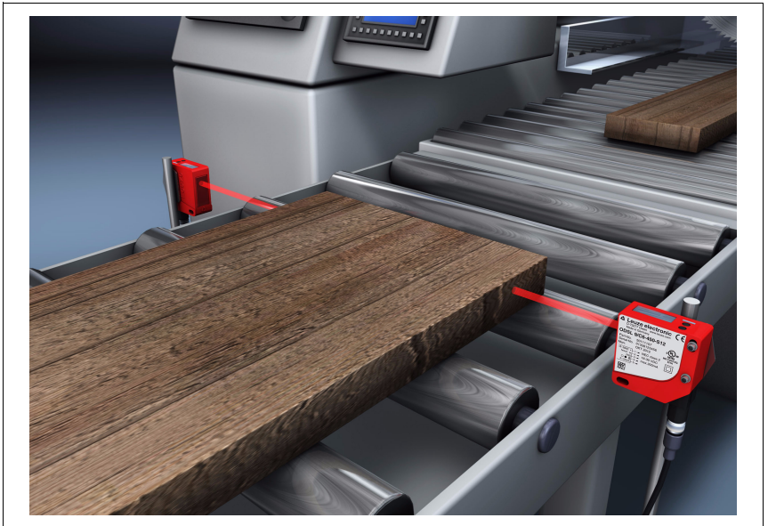
Bild 4.2: Application example: wood width measurement with the ODSL 9
