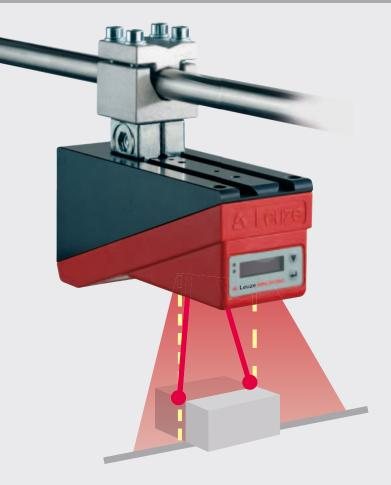
The LES sensors determine the dimensions and position of objects via their edges. By detecting height differences the sensor calculates and transfers accurate object positions. That way heights and widths or positions are reliably provided as data for further processing. At the same time one or more edge positions can be output via the individual configuration.
