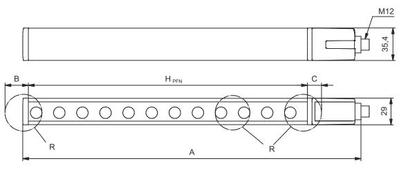
$H_{\mathsf{PFE}}$  Effective protective field height = 1228 mm  $H_{\mathrm{PFN}}$  Nominal protective field height = 1200 mm
