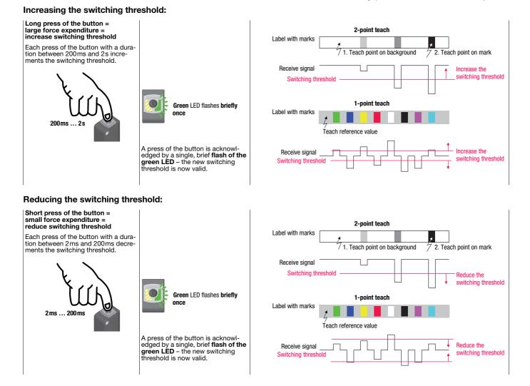
If the upper or lower end of the adjustment range is reached, the green and yellow LEDs flash at a considerably higher frequency of 8Hz for the duration of one second.
