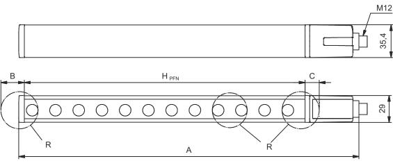
$H_{\mathrm{PFE}}$  Effective protective field height = 690 mm  $H_{PFN}$  Nominal protective field height = 600 mm
