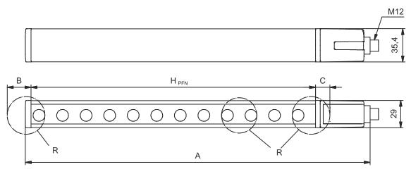
$H_{\mathsf{PFE}}$  Effective protective field height = 328 mm  ${\rm H_{PFN}}$  Nominal protective field height = 300 mm
