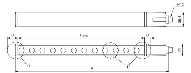
$H_{\mathsf{PFE}}$  Effective protective field height = 1812 mm  ${\rm H}_{\rm PFN}$  Nominal protective field height = 1800 mm
