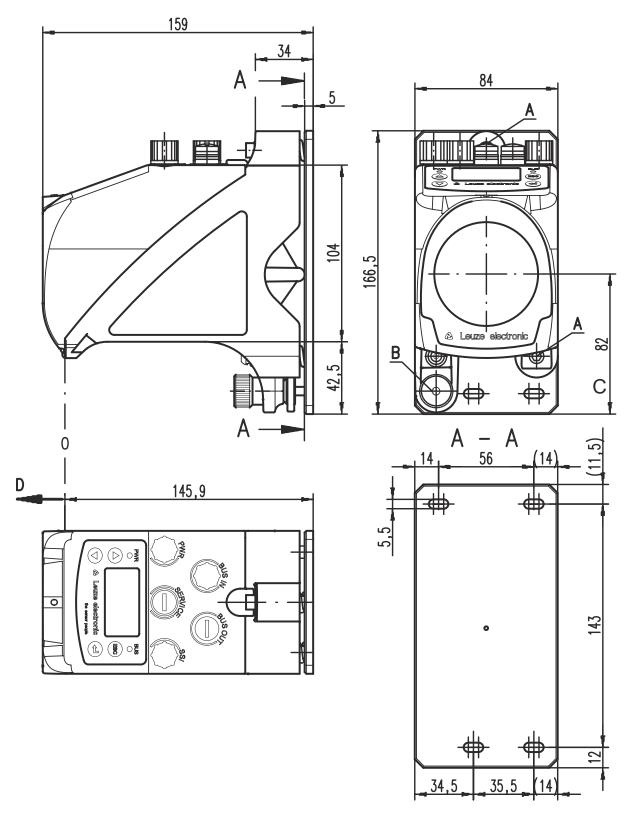
A M5 screw for alignment
