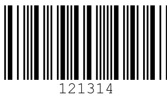
Figure 17.15: Code type 11: Codabar
