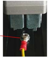
All devices can also be connected to ground potential at the M4 threaded hole on the dovetail.
