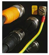
Devices produced after April 2011 are equipped with an additional grounding terminal.
