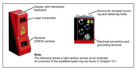
Figure 4.1: Mechanical design of Leuze light section sensors
