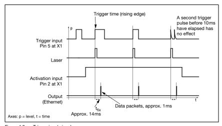
Figure 4.3: Trigger input signal sequence
