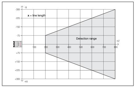
Figure 14.1: Typical detection range LRS
