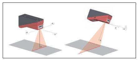
Figure 5.6: Alignment to the measuring plane
