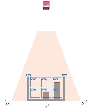
Figure 4.8: Single or multiple track presence control on transport systems
