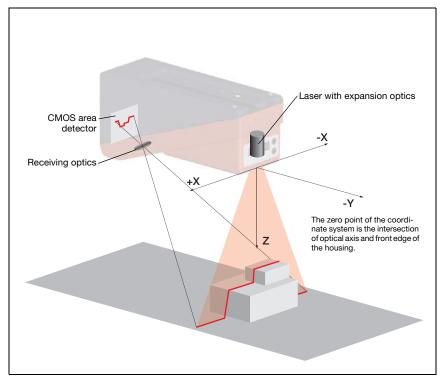
Figure 3.1: Light section sensor design
