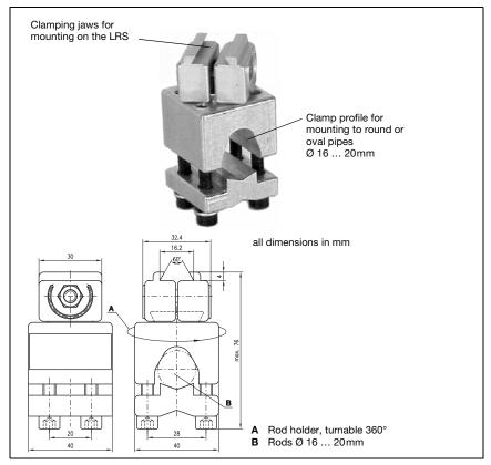
Figure 5.4: BT 56 mounting device
