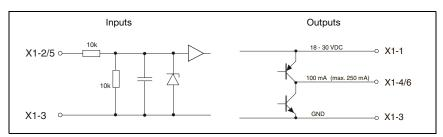
Figure 6.6: Internal wiring at X1
