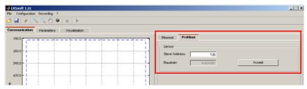
Figure 11.1: PROFIBUS address assignment with LRSsoft
