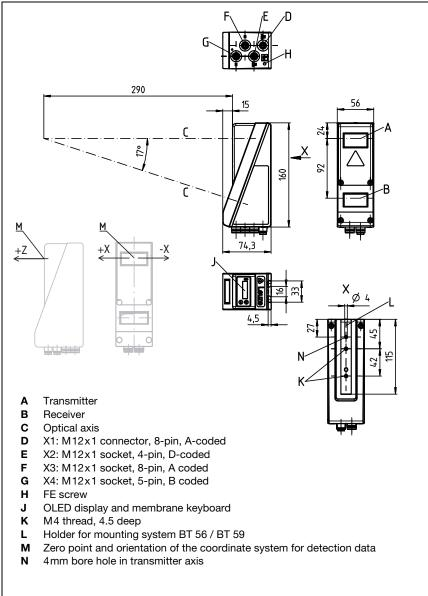
Figure 14.2: LRS dimensioned drawing
