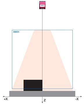
Figure 4.10: "Area Scan" teach (Area Scan Basic) - object detection in AW01
