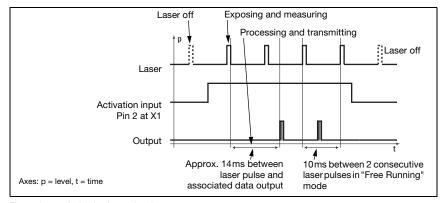
Figure 4.2: Activation input signal sequence
