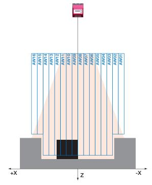
Figure 4.12: "Background Suppression" teach (Area Scan Advanced) - object detection in the AWs
