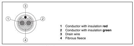
Figure 15.1: Cable structure for PROFIBUS connection cables
