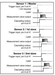
Figure 4.4: Signal sequence for cascading
