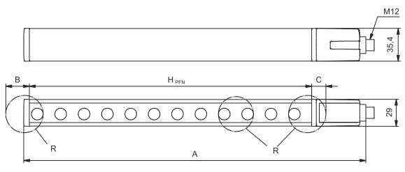
$H_{\mathrm{PFE}}$  Effective protective field height = 790 mm  $H_{\mathrm{PFN}}$  Nominal protective field height = 750 mm
