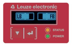
Figure 8.2: Display showing an optimally aligned light curtain
