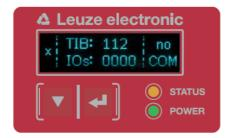
Figure 3.6: Function buttons on the receiver
