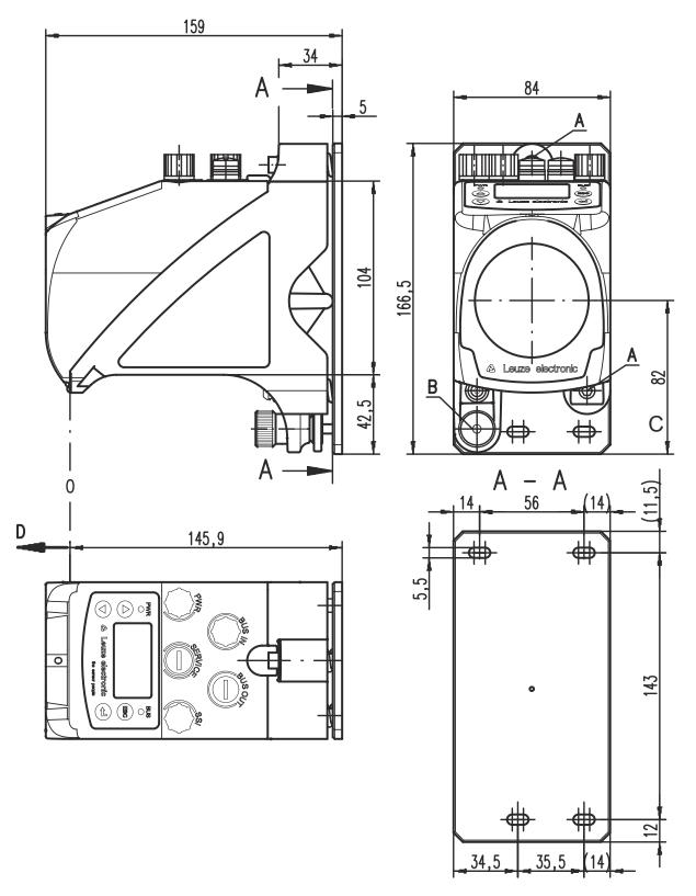
A M5 screw for alignment
