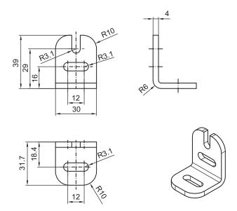
Fig. 14.4: BT-L mounting bracket
