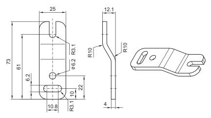
Fig. 14.5: BT-Z parallel bracket
