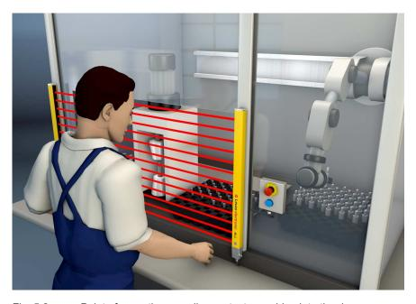
Fig. 5.2: Point of operation guarding protects reaching into the danger zone, e.g. for a pick & place robot application
