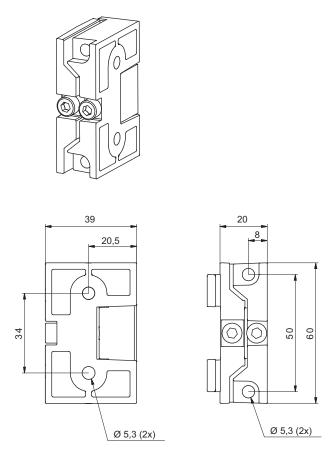
Fig. 14.7: Swiveling mounting bracket BT-2SB10
