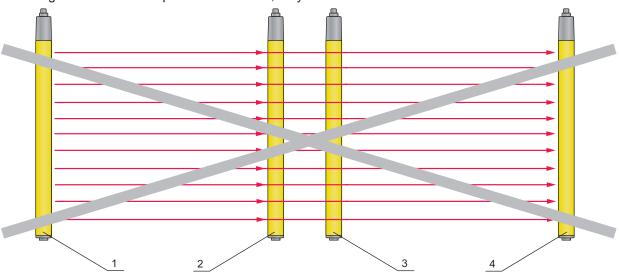
Fig. 6.4: Optical crosstalk between adjacent safety sensors (transmitter 1 influences receiver 2) due to incorrect mounting
