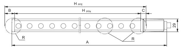
Fig. 14.1: Dimensions of Host transmitter and Host receiver
