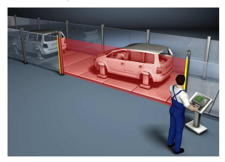
Fig. 5.3: Access guarding on a transfer path
