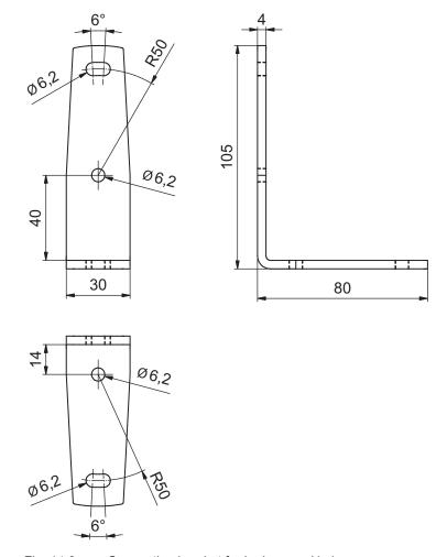
Fig. 14.8: Connection bracket for L-shape or U-shape
