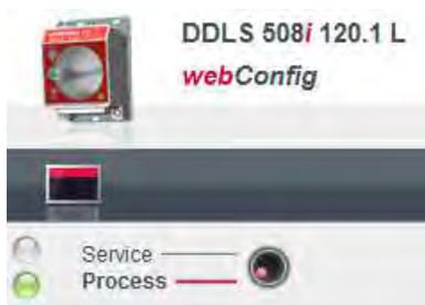
Fig. 8.4: Changing the operating mode (Process - Service)
