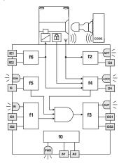
The "RUN" operating state indicates normal operation: Function f1 evaluates the state of the IS1 and IS2 inputs, while at the same time function f2 checks that the actuator is present, and function f4 checks that the actuator has been locked.
