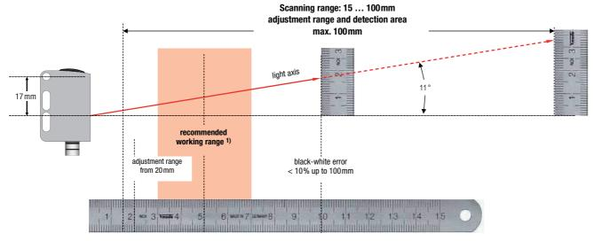
1) The sensor is most capable of reliably detecting a reflective surface or transparent object in the recommended working range. Nevertheless, the sensor can reliably detect such objects in the entire scanning range; however, the performance reserve is reduced as compared with the recommended working range.
