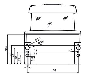
Minimum space requirements for installation and replacement of scanner unit
