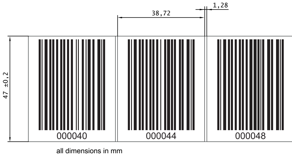
Figure 13.12: Dimensioned drawing bar code tape BCB with 40 mm grid
