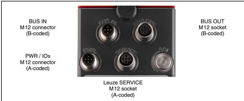
Figure 7.1: Connections of the AMS 301 i
