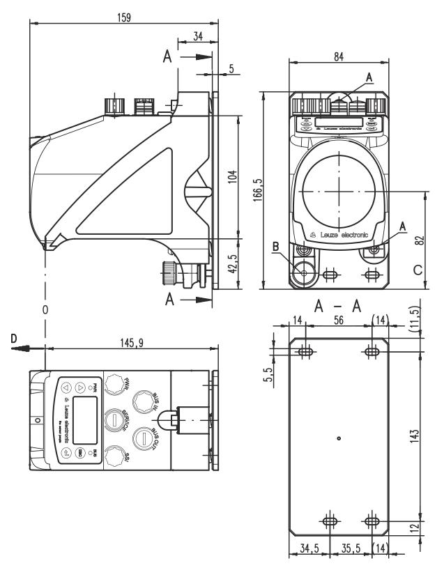
A M5 screw for alignment
