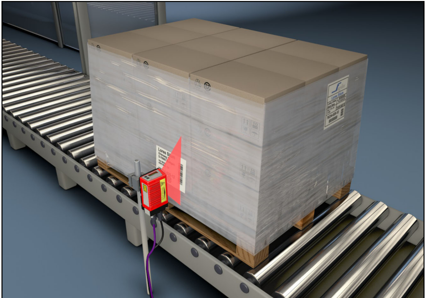
Figure 4.8: Deflection principle for the line scanner
