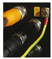
Devices produced after April 2011 are equipped with an additional grounding terminal.
