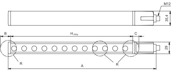
$H_{\mathsf{PFE}}$  Effective protective field height = 312 mm  ${\rm H_{PFN}}$  Nominal protective field height = 300 mm
