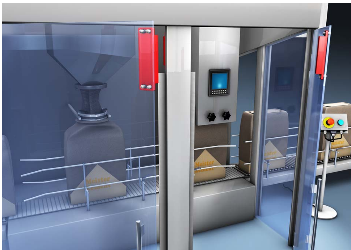
Figure 5.2: Access guarding on a filling system, realized on a door with MC388x sensors
