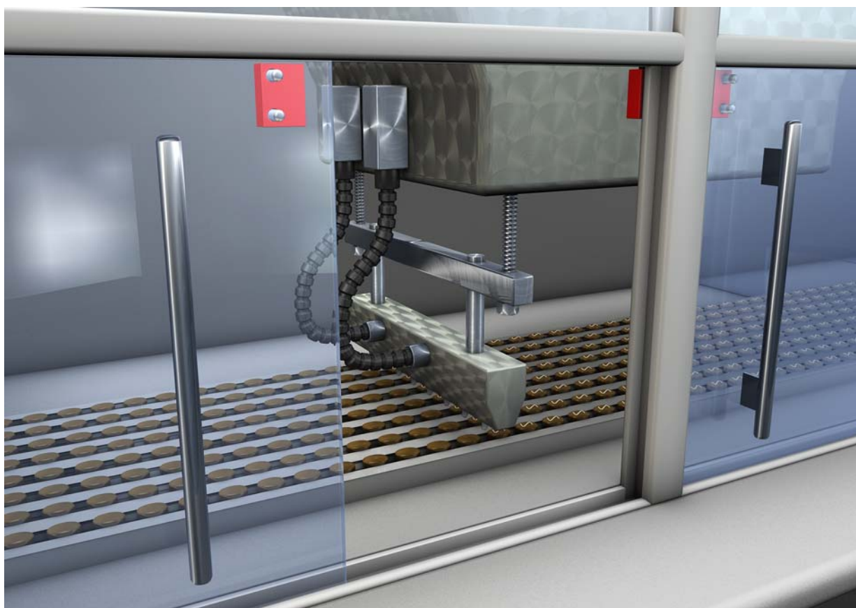
Figure 5.4: Access safeguarding on a food production line, implemented on a sliding gate with MC336x sensors
