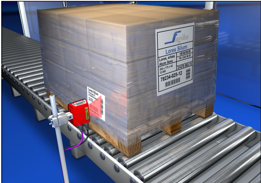
Figure 4.4: Deflection principle for the line scanner
