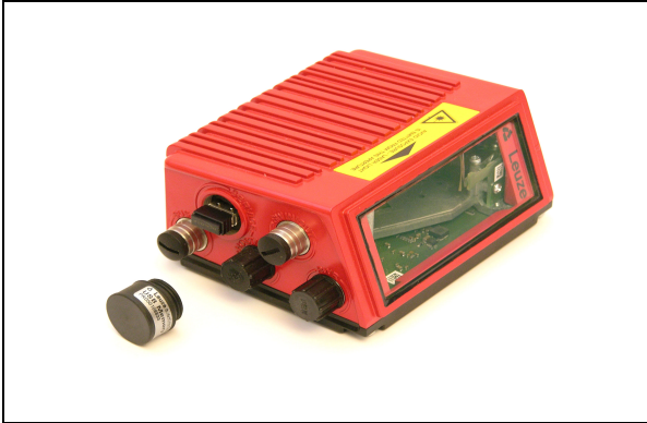
Figure 10.19: Installing the external parameter memory
