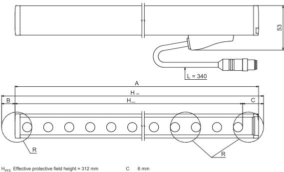
$H_{PFN}$  Nominal protective field height = 300 mm
