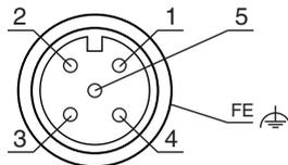
Fig. 7.1: Pin assignment transmitter
