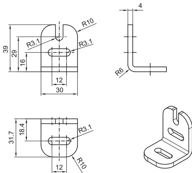
Fig. 14.2: BT-L mounting bracket
