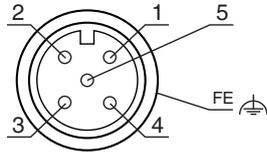
Fig. 7.2: Pin assignment receiver
