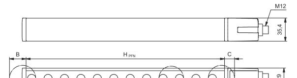
$H_{\mathsf{PFE}}$  Effective protective field height = 478 mm  $H_{\mathsf{PFN}}$  Nominal protective field height = 450 mm
