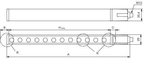
$H_{\mathsf{PFE}}$  Effective protective field height = 2340 mm  $H_{\mathrm{PFN}}$  Nominal protective field height = 2250 mm
