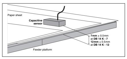
Figure 4.3: Mounting the capacitive sensor
