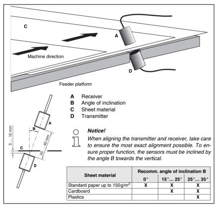
Figure 4.2: Mounting the ultrasonic sensors
