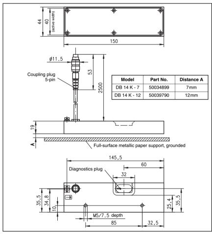
Figure 9.2: Capacitive sensor DB 14 K
