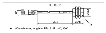
Figure 9.3: Ultrasonic transducer DB 18 UP
