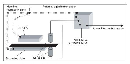
Figure 4.4: Potential equalisation and connection
