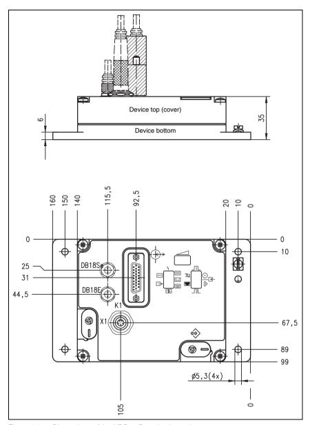
Figure 9.1: Dimensions of the VDB 14B evaluation unit
