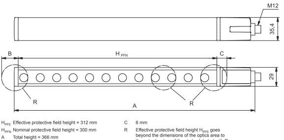
В 6 mm Effective protective field height H<sub>PFE</sub> goes beyond the dimensions of the optics area to the outer borders of the circles labeled with R.
