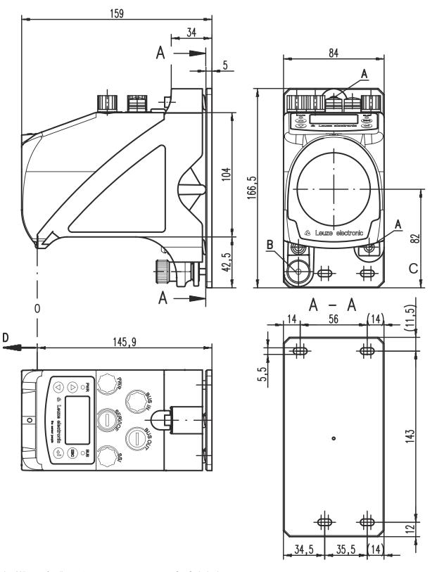
A M5 screw for alignment
