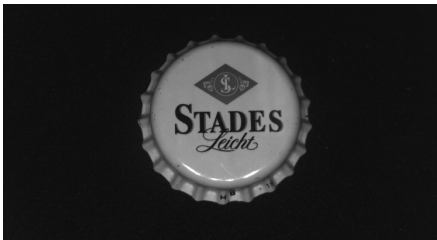
Figure 4.59: Inclined camera alignment with only three illumination quadrants active (reflected quadrant is off) - nearly all reflections in the image are suppressed
