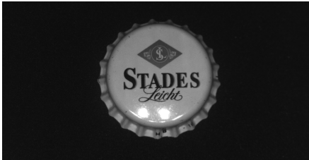
Figure 4.58: Inclined camera alignment with all four illumination quadrants active - better, but reflections still visible in one quadrant
