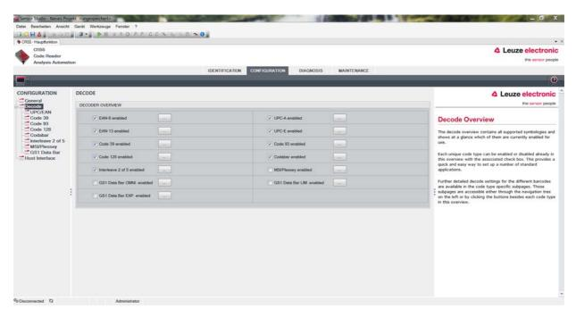
Figure 6.4: Decode tab
