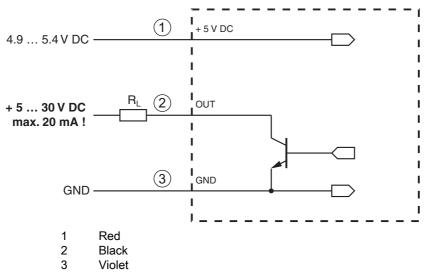
Figure 5.2: Switching output
