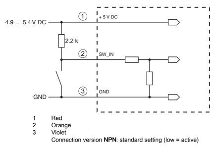
Figure 5.1: Wiring example of the trigger input
