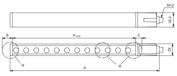
$H_{\mathrm{PFE}}$  Effective protective field height = 912 mm  $H_{\mathrm{PFN}}$  Nominal protective field height = 900 mm
