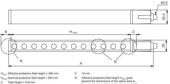
В 25 mm Effective protective field height H<sub>PFE</sub> goes beyond the dimensions of the optics area to the outer borders of the circles labeled with R.
