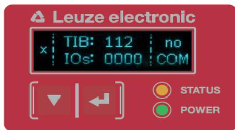
Figure 3.3: OLED display on the receiver
