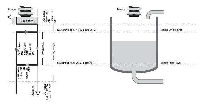
If the container is empty, e.g. after a cleaning or an initial filling, the sensor must first send an active control signal for a pump which fills the container up to the maximum fill level.
