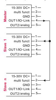
In contrast to multiplex operation, addressing of the sensors is unnecessary.
