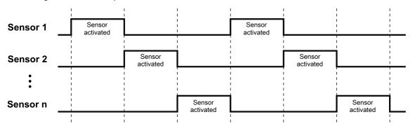
**NOTE** With the min. activation time, the sensor operates faster, but also with a low analysis depth. If a high functional reliability is required, we recommend doubling the activation time.
