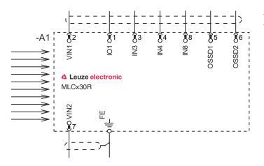
• VIN1 = +24 V, VIN2 = 0 V: transmission channel C1
