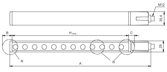
$H_{\mathsf{PFE}}$  Effective protective field height = 2740 mm  $H_{\mathrm{PFN}}$  Nominal protective field height = 2700 mm
