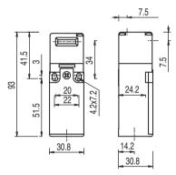
Figure 3.1: Dimensions of S20-P3C1-M20-FH, S20-P1C1-M20-FH30 and S20-P4C1-M20-FH in mm
