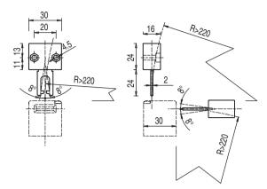
Figure 13.3: AC-AN-F4 actuator
