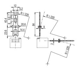
Figure 13.5: AC-AN-SL actuator
