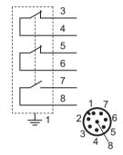
Figure 7.4: Pin assignment of the 8-pin M12 plug (S20-xxx-M12-xxx)
