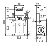
Figure 3.3: Dimensions of S20-P1C3-M20-LH and S20-P4C3-M20-LH in mm
