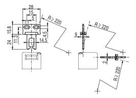
Figure 13.1: AC-AN-S actuator
