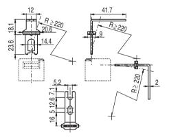
Figure 13.6: AC-AN-AL actuator
