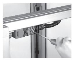
♥ Tighten the housing cover with 0.7–0.9Nm.
