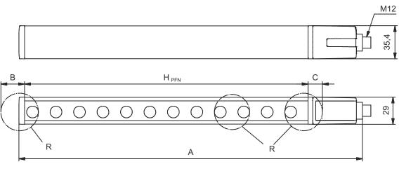
$H_{\mathsf{PFE}}$  Effective protective field height = 2712 mm  ${\rm H}_{\rm PFN}$  Nominal protective field height = 2700 mm
