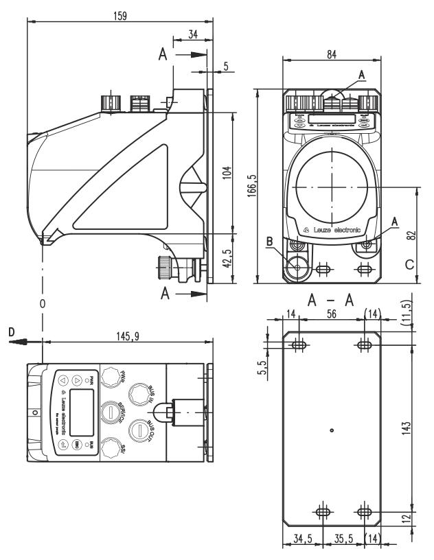
A M5 screw for alignment
