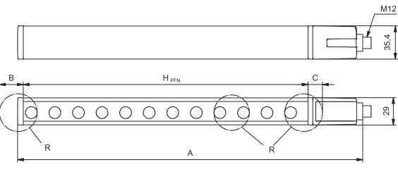
$H_{\mathsf{PFE}}$  Effective protective field height = 2412 mm  ${\rm H}_{\rm PFN}$  Nominal protective field height = 2400 mm
