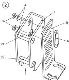
2.Fit fastening screws (item 3) with washers (item 4) according to diagrams ①, ①, ① depending on the installation situation, push through the device and securely tighten.
