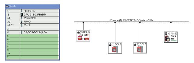
Fig. 7.2: PROFINET topology with DDLS 548i in the hardware configuration
