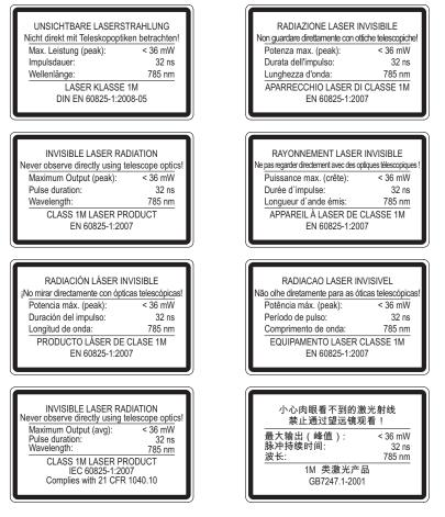
Fig. 2.2: Laser warning and laser information signs for devices with frequency F3
