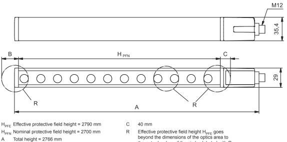
В 50 mm Effective protective field height H<sub>PFE</sub> goes beyond the dimensions of the optics area to the outer borders of the circles labeled with R.
